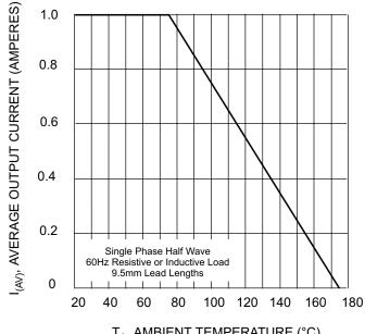
T<sub>A</sub>, AMBIENT TEMPERATURE (°C) Fig. 1, Forward Current Derating Curve
